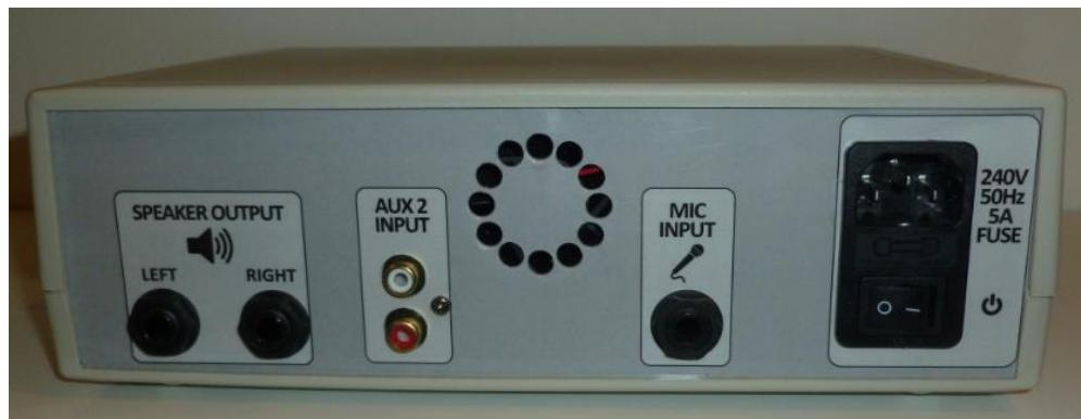
2. Connect the kettle lead to the socket at the back of the amplifier (top right socket labelled 240V). Switch on using the rocker switch at the back of the amplifier (bottom right). The power indicator light on the front of the amplifier should light up (bottom right hand corner of the front of the amplifier).
