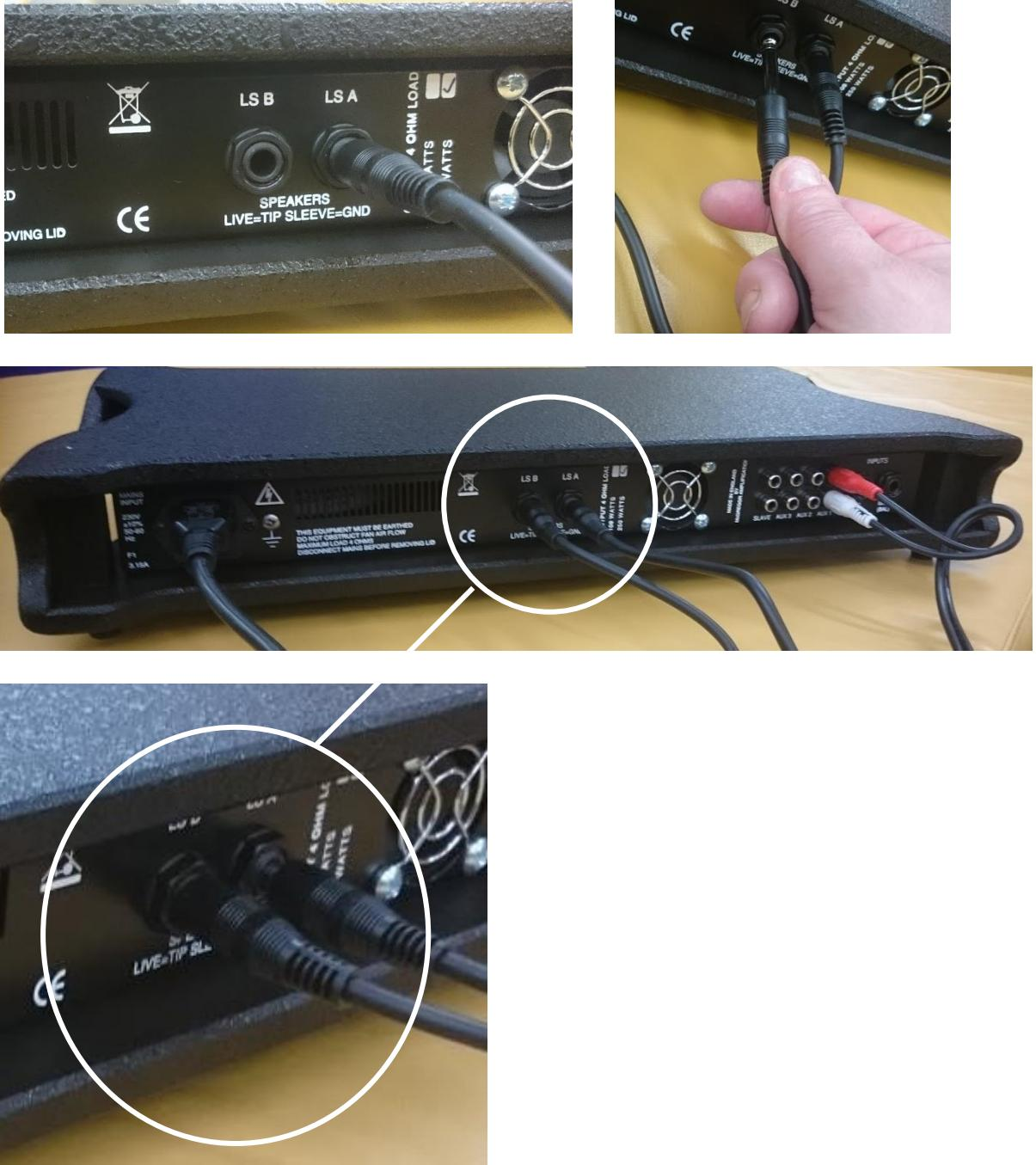
It does not really matter which end of the “Speaker to Amplifier” lead fits into the jack socket place, however, we recommend that the shorter, black angle jack plugs (A) are connected to the base of the Water Mattress to enable it to fit flush against a wall.
